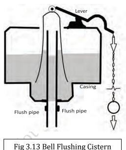
chain should be released immediately after being pulled to force the water out of the flush pipe. This cistern is supplied with water through a ball valve arrangement. The water inlet closes
