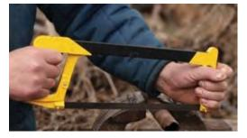
Fig 2.3 Cutting with a hacksaw
